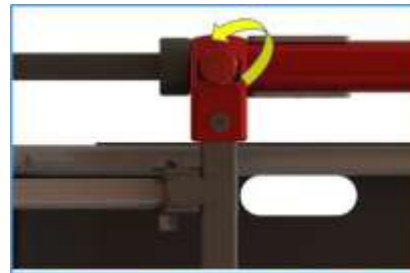
Rotate the conversion lock 90°
